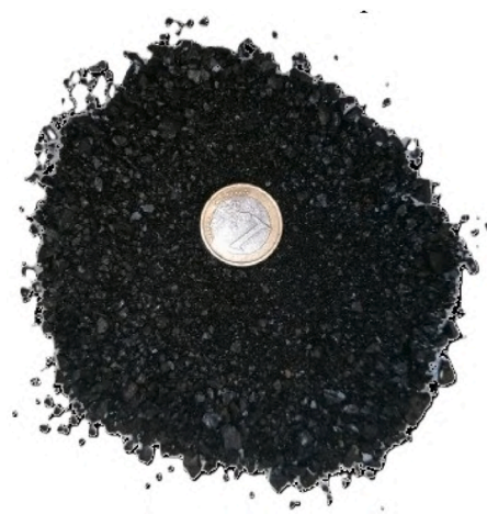
Fig. 1. A sample of SNB used for the production of bituminous blends.
