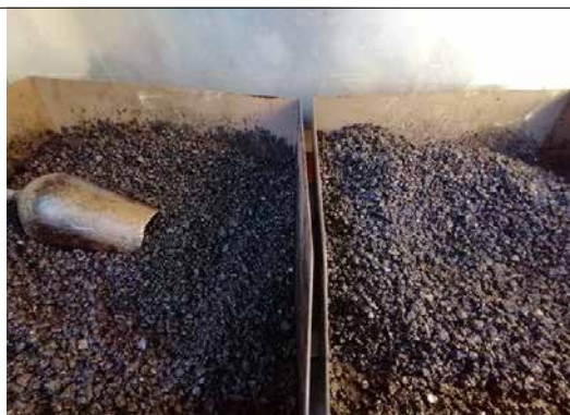
3. Conglomerati bituminosi in cella climatica a 40 °C
