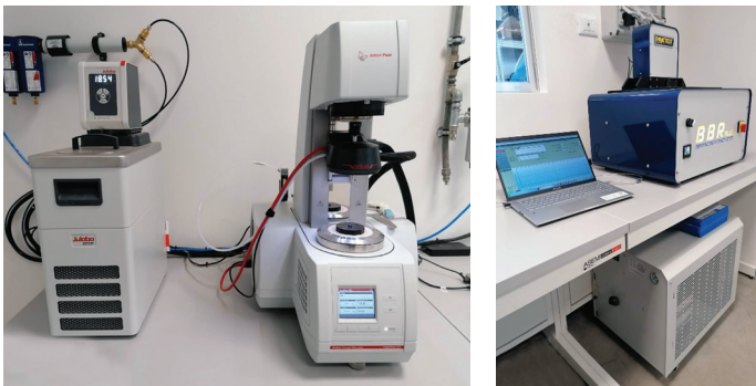
10A e 10B. Il Dynamic Shear Rheometer (DSR) e il Bending Beam Rheometer (BBR)
