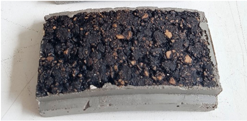
Figure 4. Curved HMA samples for skid resistance evolution measurements.
